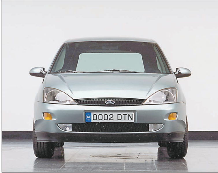
This 1999 Focus was the first car to have a plastic metal hybrid bumper.
