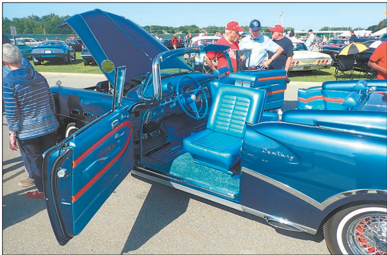
The 1956 Buick X came with swivel driver and front passenger seats.
