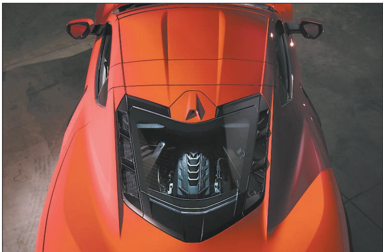
The new Stingray has a mid-engine design – a first for the Corvette.
