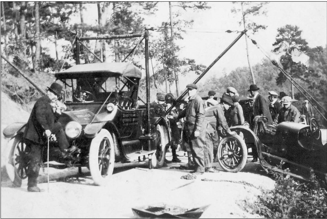
The first tow truck, seen here pulling a car out of a ditch, was actually built on a Cadillac body in 1916.
