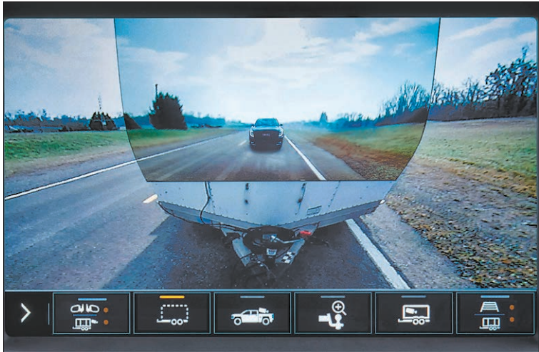
A camera makes it possible to see behind the trailer being towed.
