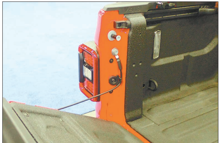
A simple cable lets the Gladiator tailgate be open in different positions.
