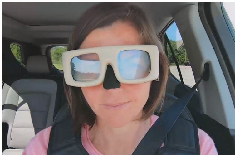
This geat used by a GM engineer recreates the effects of drowsy driving.
