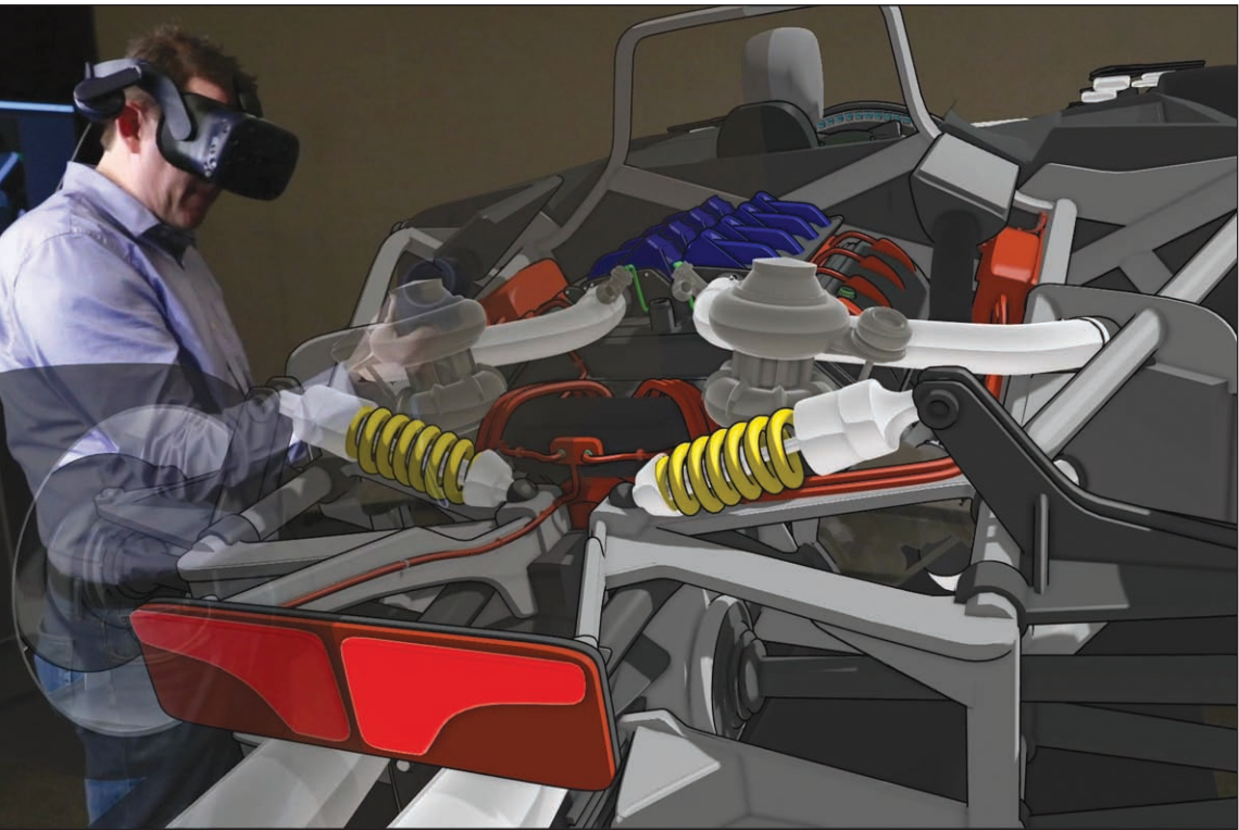
Ford's the first OEM to use Gravity Sketch – a 3D virtual reality tool that helps design human-centric vehicles.
