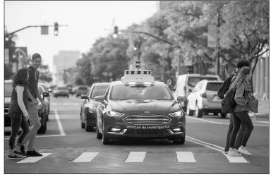
**CONTINUED ON PAGE 6** The Ford light bar uses three light signals to indicate vehicle status.
