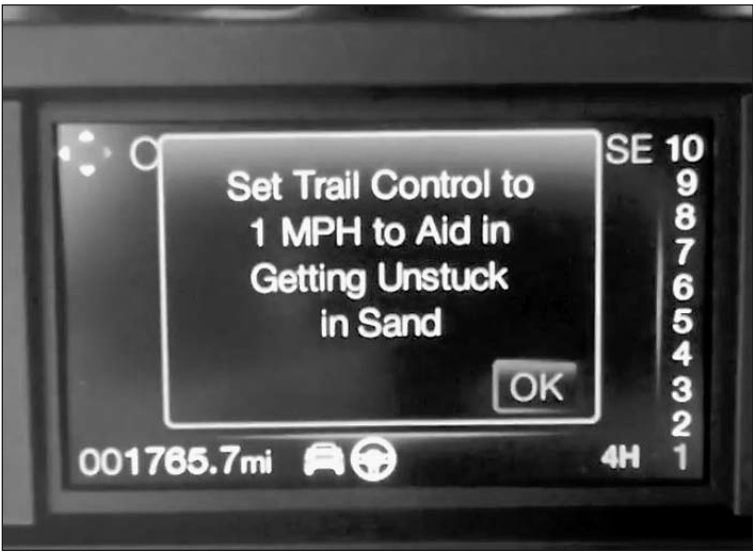
To get unstuck, Trail Control can be activated from 1 mph up to 20 mph.
