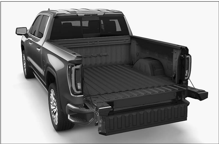
2019 Sierra Denali’s tailgate can be configured into different shapes.
