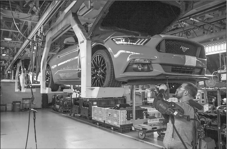
Ford’s EksoVest is used to reduce the physical toll on employees.
