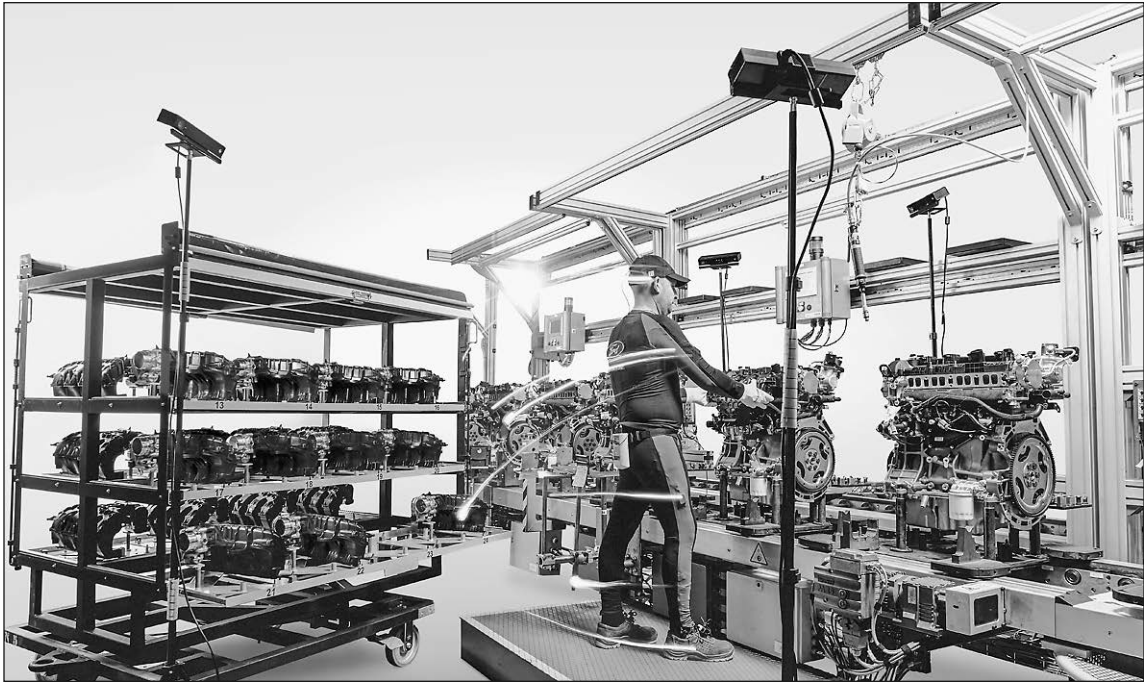
Body tracking technology is being used to improve auto assembly line production at a Ford plant in Spain.
