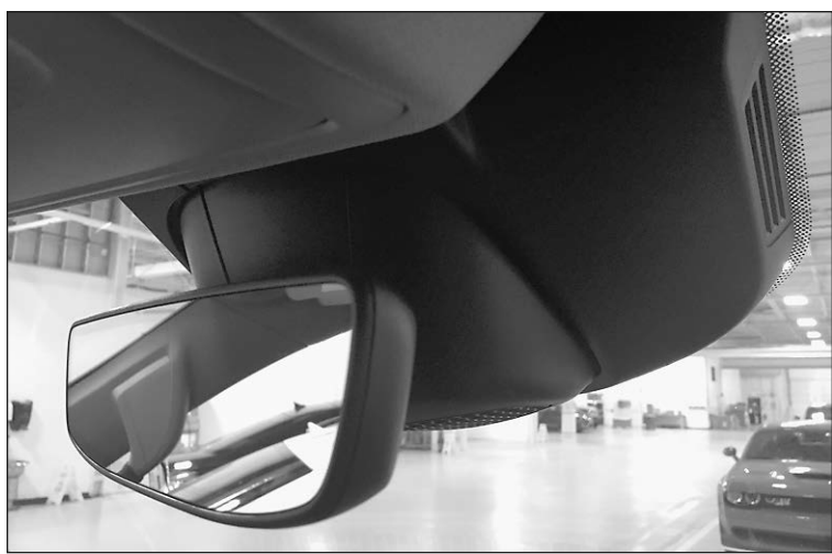
Camera, radar for AEB integrated safety system in the 2019 Ram 1500.
