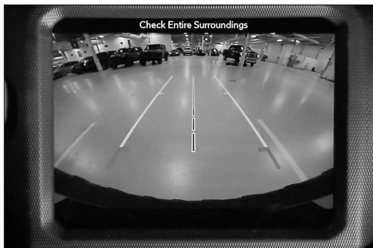
A view of the guide lines in FCA's new rear-view camera system.
