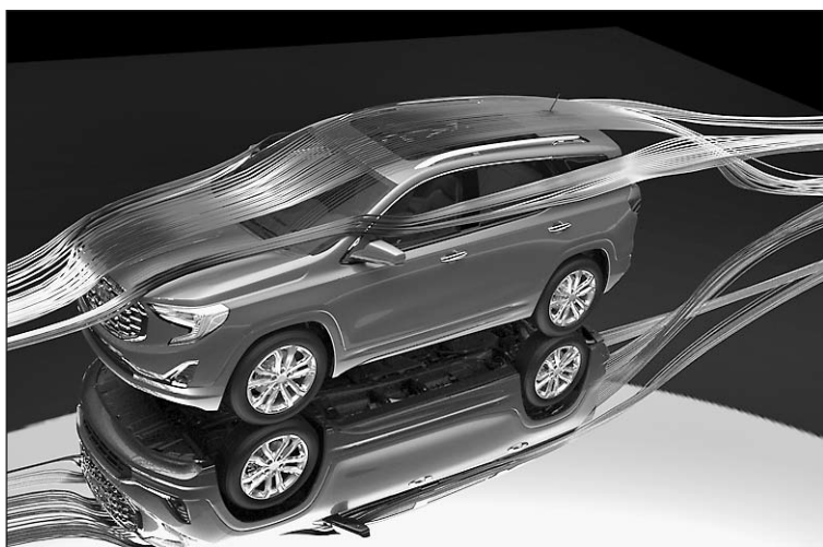
GMC aerodynamicists use fluid dynamic tools to test airflow.
