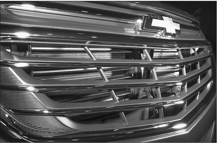
Controlled upper, lower grille shutters improve Equinox aerodynamics.
