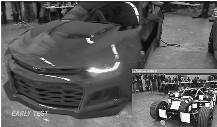
The “skin” of the vehicle is added digitally via computer technology.
