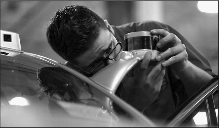
Ford employee instals new LiDAR to test an autonomous Fusion hybrid.
