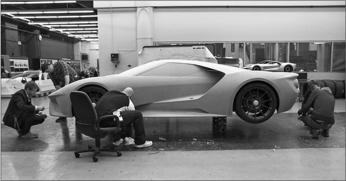
Clay is still used in Ford's design process, and the company has found ways to recycle it for further use.
