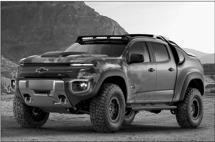
Fuel-cell-powered electric Chevrolet Colorado ZH2 test vehicle
