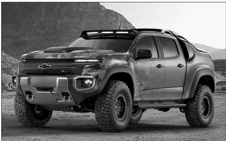
Fuel-cell-powered electric Chevrolet Colorado ZH2 test vehicle
