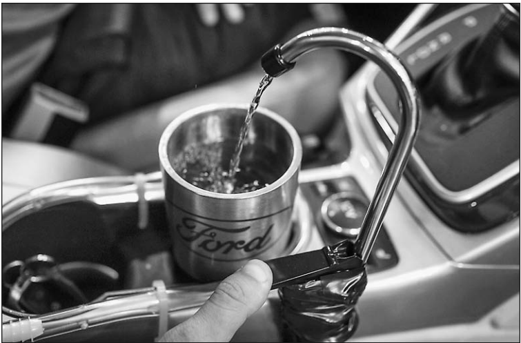
On-the-Go H2O system collects, filters and pumps water to cupholders.
