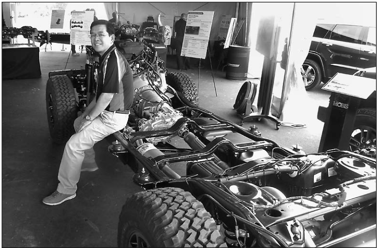
Jimmy Park with a Mobis-made chassis for a Jeep Wrangler.
