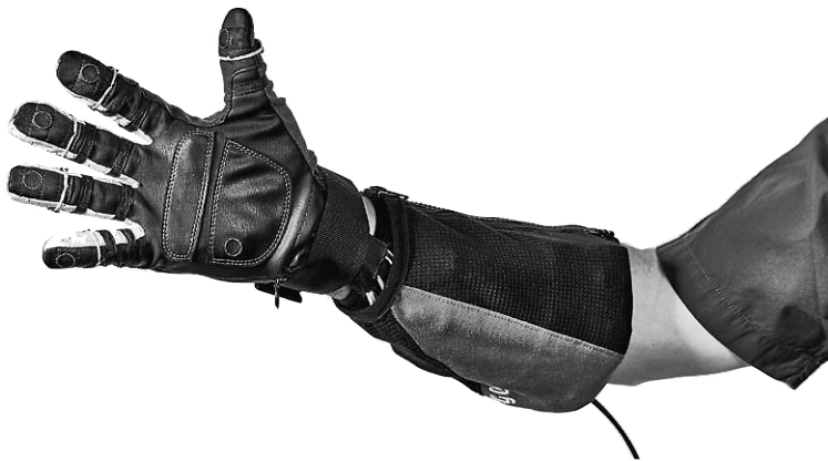
GM's new RoboGlove enhances a user's hand strength in manufacturing.
