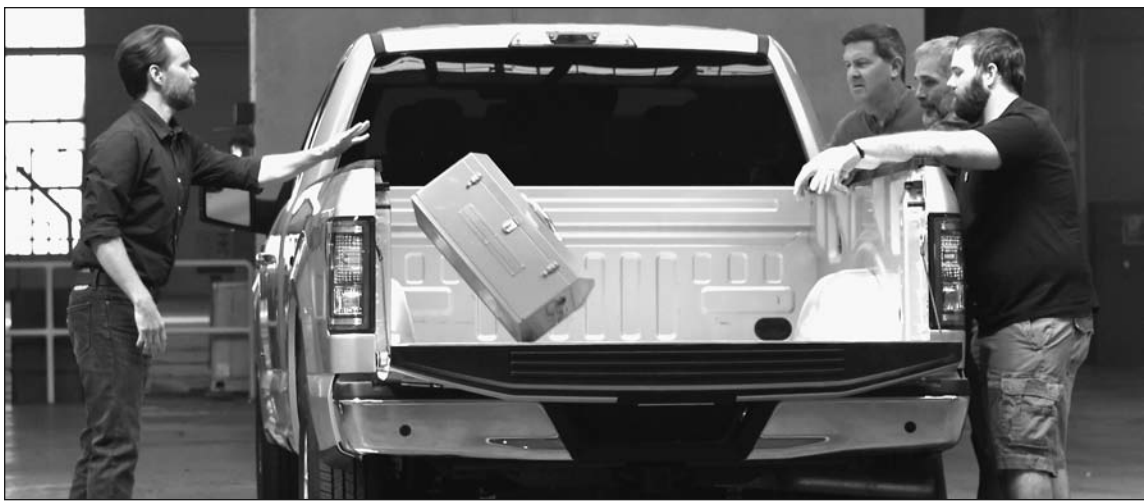
GM tests comparable pickups as 28-pound toolboxes are dropped into the beds of Silverados and F-150s.
