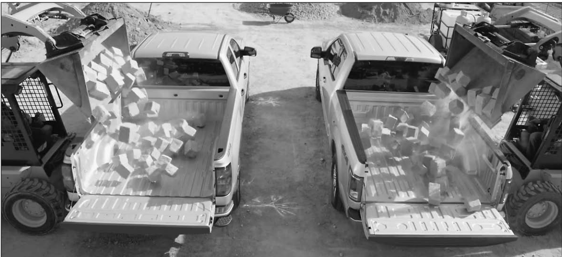
GM tested the beds of Silverado, left, and F-150 pickups by dropping landscaping blocks from five feet.
