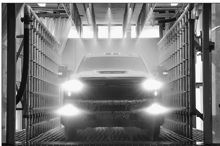
Silverado air scoop runs through "driving rain" simulated test.
