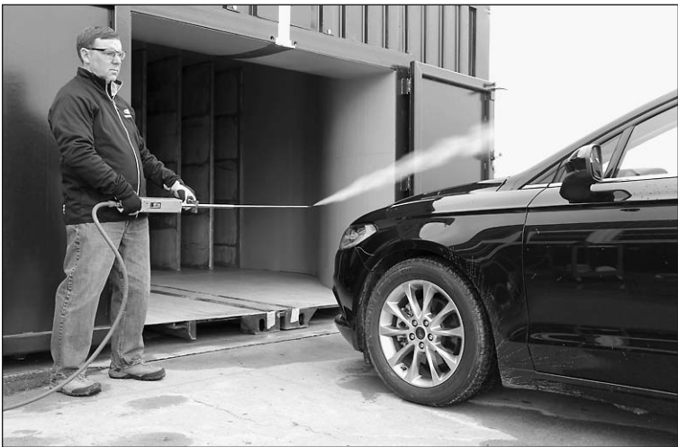
Ford engineer uses smoke nozzle to test a vehicle's wind noise.
