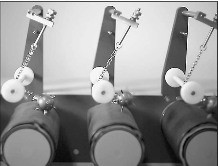
Mace Snagging Test – spinning seat fabrics by spikey iron balls.
