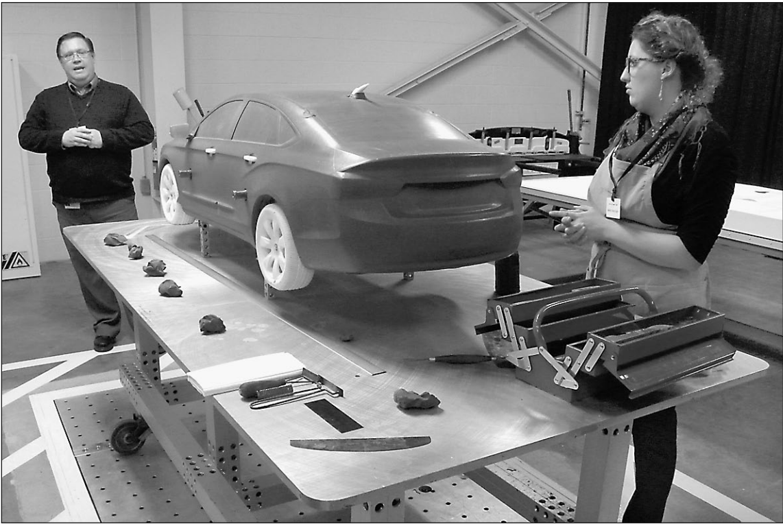
Jeff Bordner and Bailey Sisoy Isgro show how GM's reduced-scale wind tunnel sculpting table is used.
