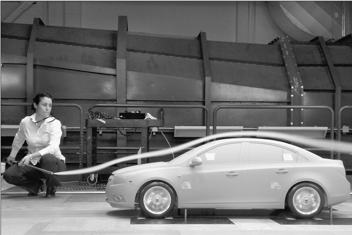
GM engineer Nina Tortosa demonstrates how aerodynamic qualities are measured in small-scale wind tunnel.
