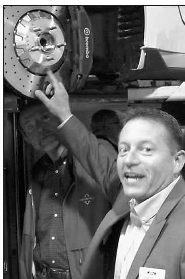
Dave Pericak points out the GT350's two-piece cross-drilled iron rotors.
