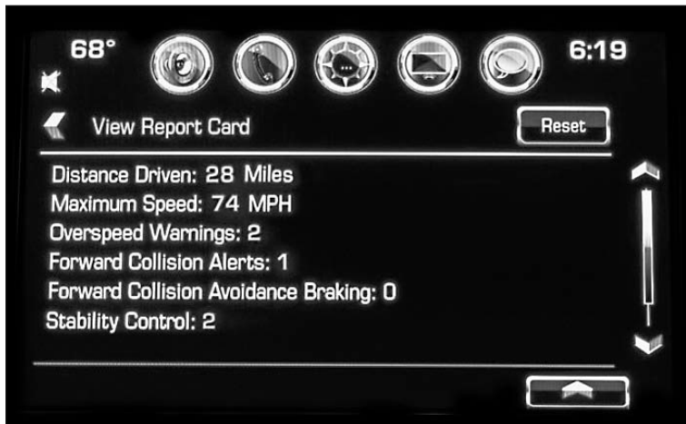
This Malibu display shows how driving safety standards are recorded.
