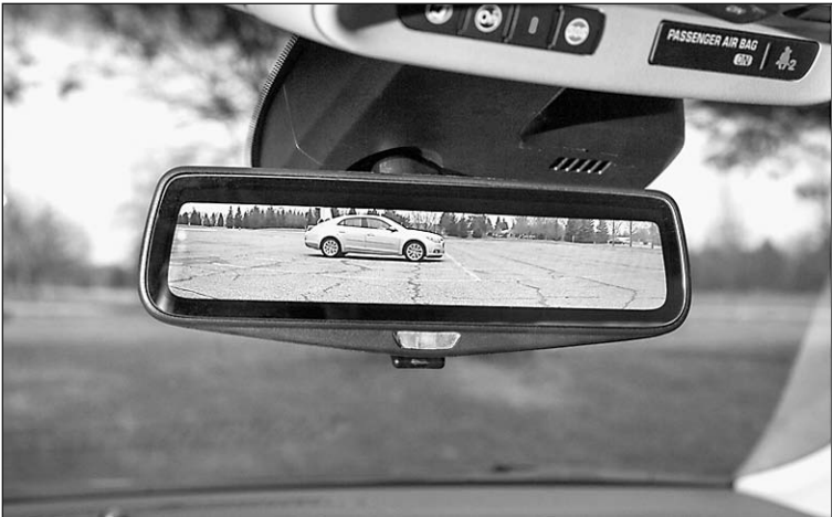
Views with the new video mirror (above) and traditional mirror (below)
