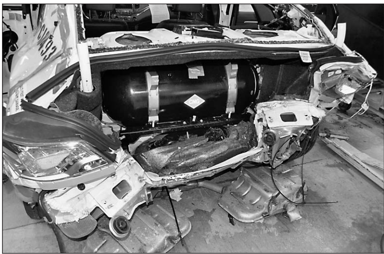
Impala's CNG tank is intact after crash test at GM Proving Ground.
