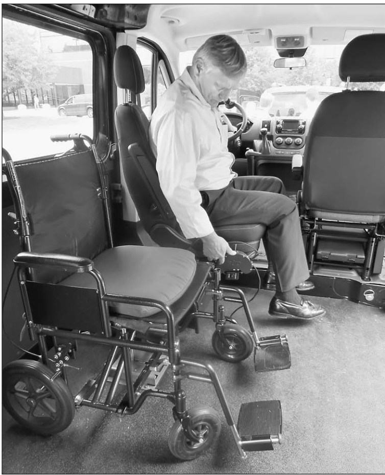
Commercial Van Product Planning Manager Mike Pultorak demonstrates how to transfer from the wheelchair to the swiveling power driver's seat in the ProMaster full-size van.
