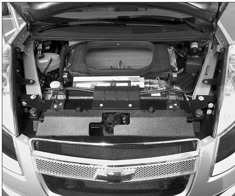
The Sequel hydrogen fuel cell fits completely under the van's hood.
