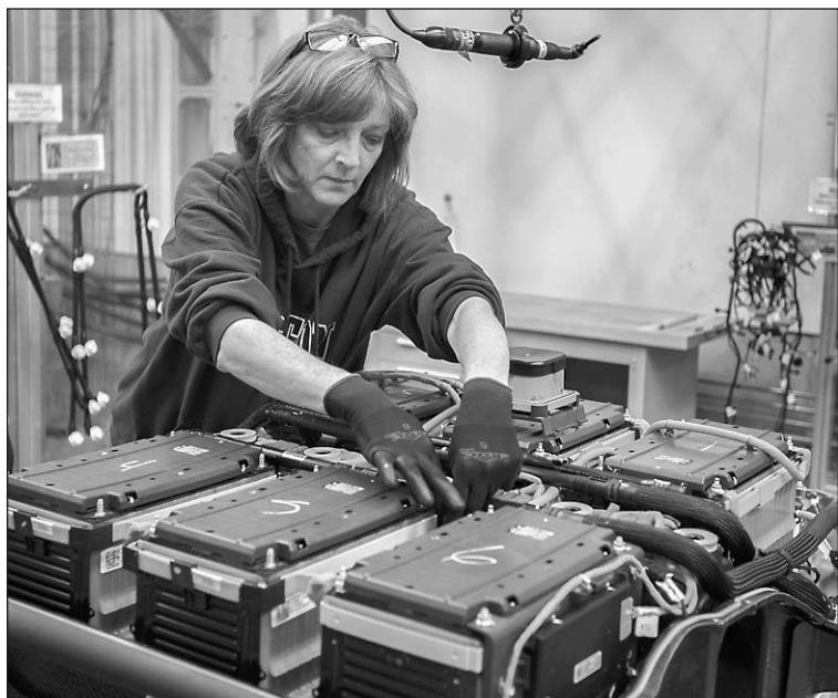
Brownstown's Tina Oaks puts wiring harnesses on a Spark EV battery.
