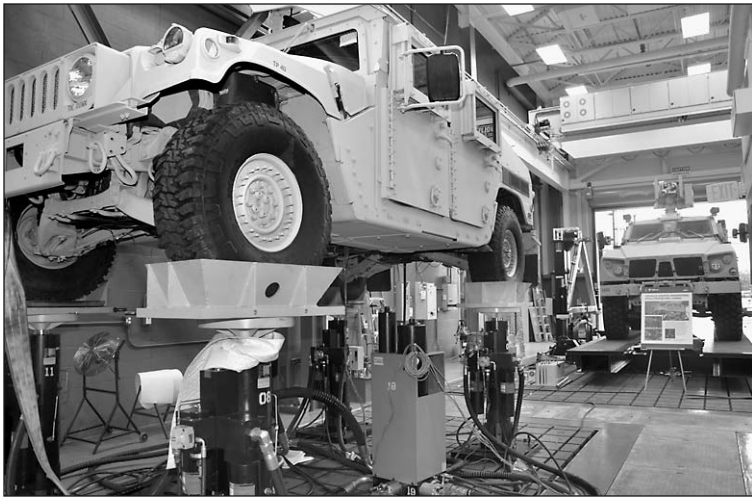
VCL test rigs can handle large vehicles weighing up to 100,000 pounds.
