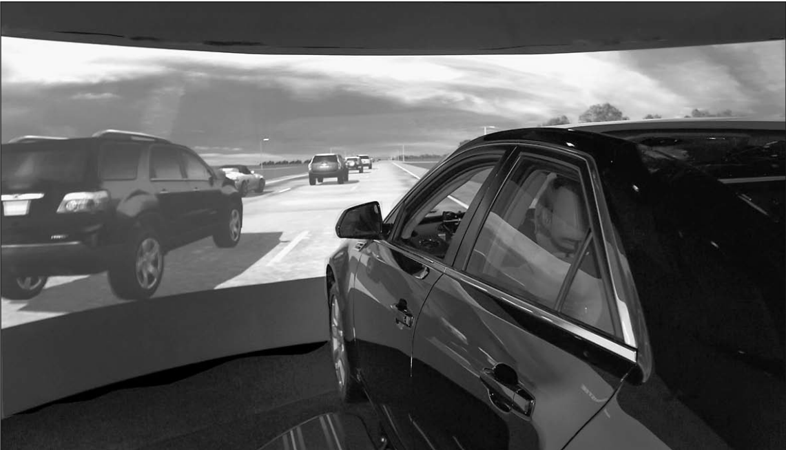
A 360-degree high-definition projection screen allows visuals to respond to steering and pedal force inputs.
