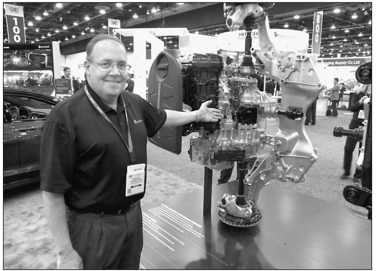
Mike Kirk shows off the 200's disconnectable driveline.
