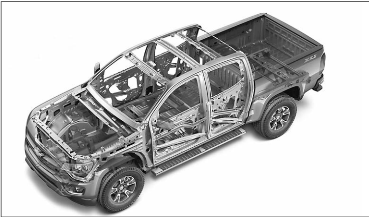
Colorado skeleton shows use of high-strength steels and aluminum.
