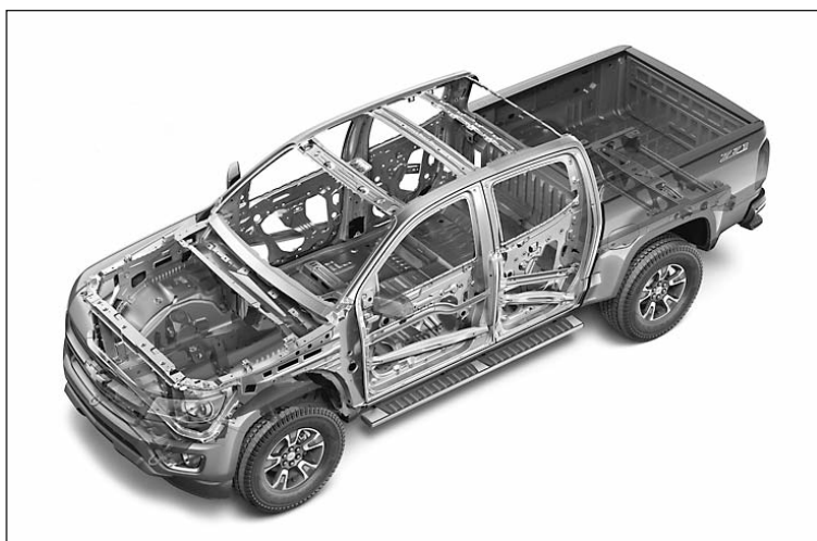
Colorado skeleton shows use of high-strength steels and aluminum.
