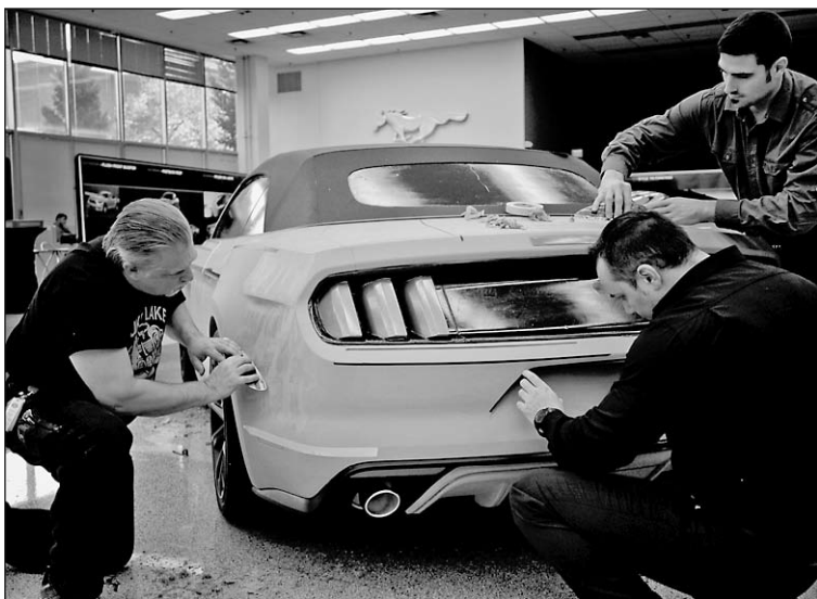
Ford still uses ordinary tape in the design process.
