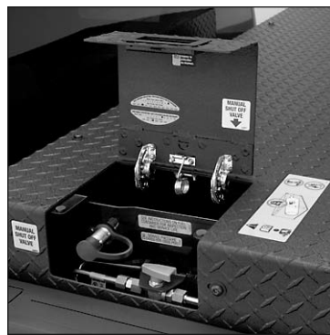
The CNG “on” switch
