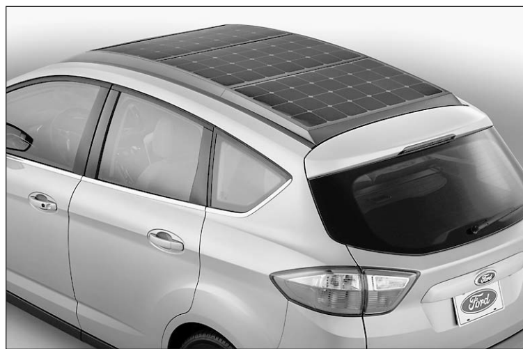
Ford is testing a C-Max that uses solar panels to produce power.
