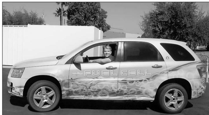
GM's test vehicle topped 100,000 'real' miles with a hydrogen fuel cell.
