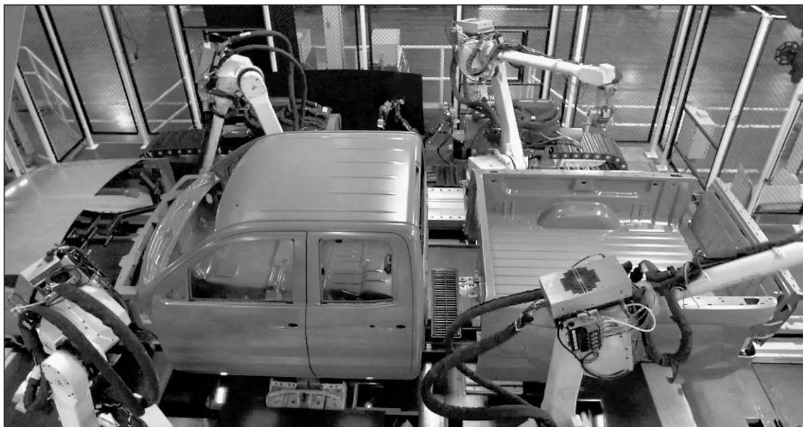
A 2014 Chevy Silverado pickup goes through the paces of hem flange sealing on doors, hood and underbody.
