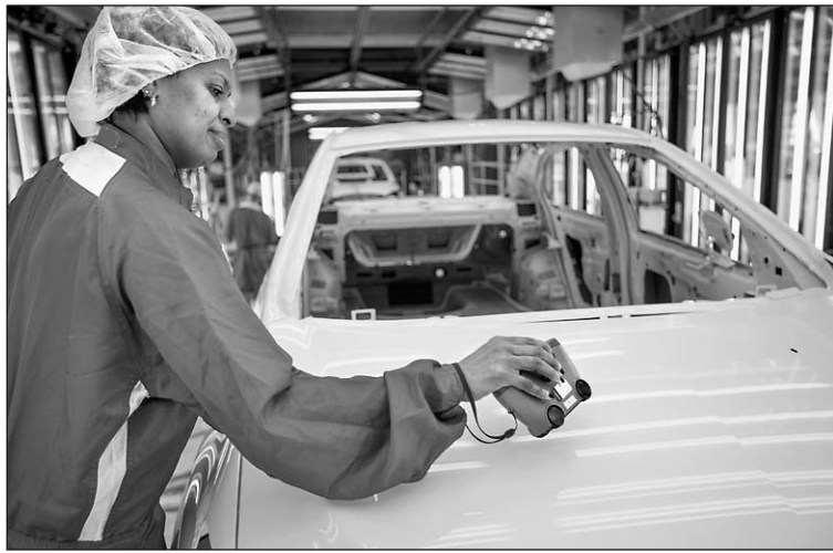
A GM worker checks for painting imperfections using a special scanner.
