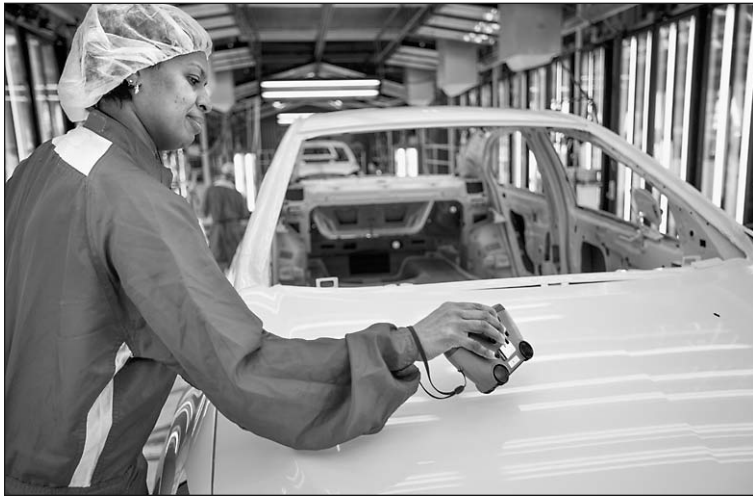
Orion Plant paint employees wear special lint-free suits for quality.
