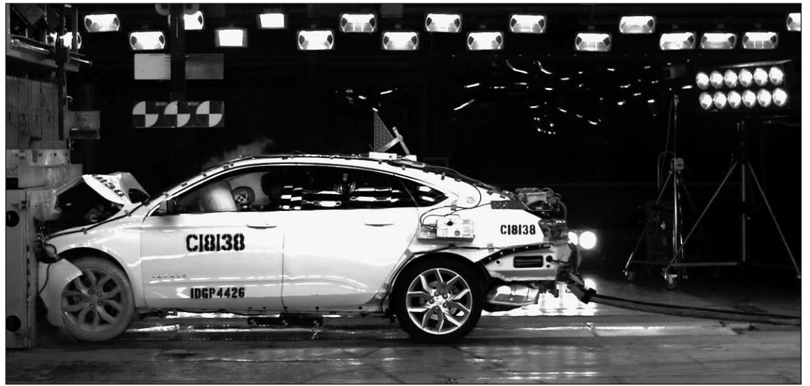
A 2014 Chevrolet Impala, which includes new safety technologies, being tested for crashworthiness.
